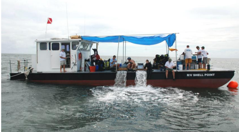
Figure 12-4. Aboard the North Carolina Marine Fisheries' barge R/V Shell Point during the 2007 QAR project. Below the surface, divers excavate two 5-foot-by-5-foot grid squares with handheld dredges. The dredged material passes through the screen/slucice boxes seen amidships. At the bow, team members process the captured sediment to extract small lead shot and gold dust.
